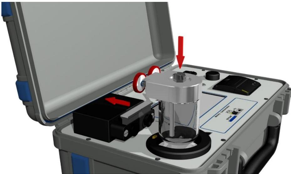
With the sliding block pushed back, position the oil container in the HYDROCAL 1011 *genX* P.
