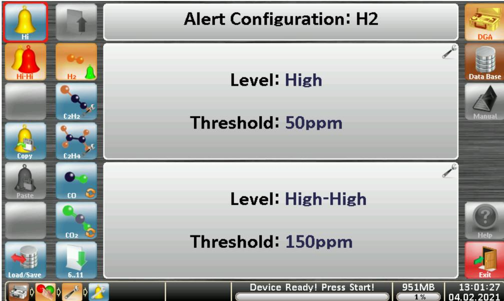
Alarm thresholds are set in the alarm configuration by pressing the respective field for the gas to be configured. Then select the Hi or Hi-Hi alarm on the left and tap on the threshold value that has not yet been set with your finger.
