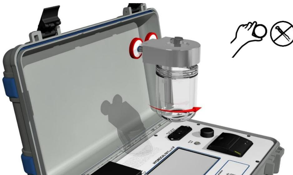
**Note:** Carefully position the thread and tighten the container by hand without using tools.
