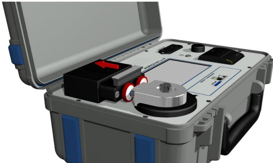
With the sliding block pushed back, pull the oil reservoir upwards out of the HYDROCAL 1011 *genX* P.
