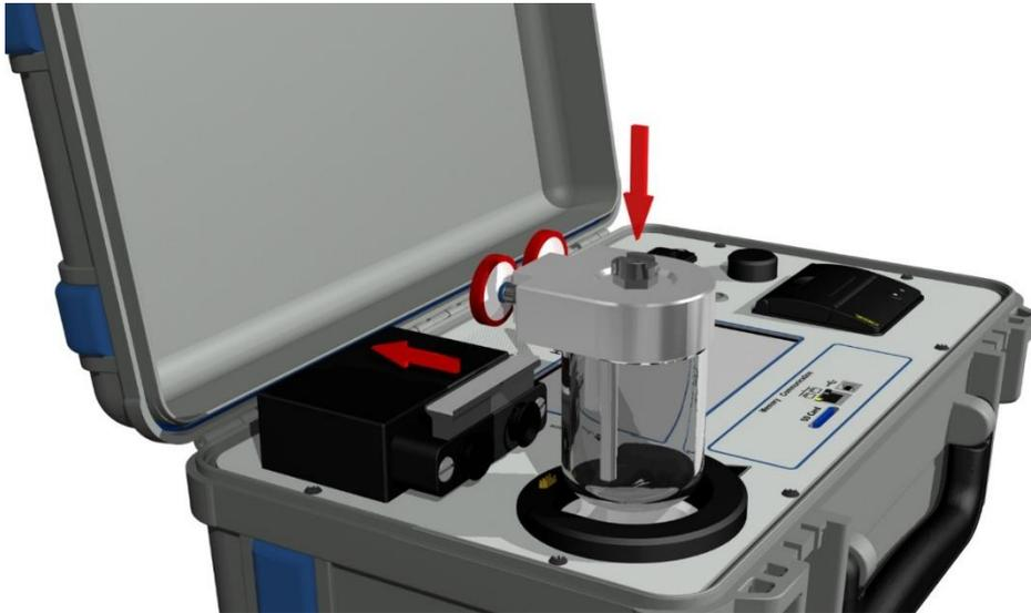
With the sliding block pushed back, put the oil container into the HYDROCAL 1011 *genX* P.
