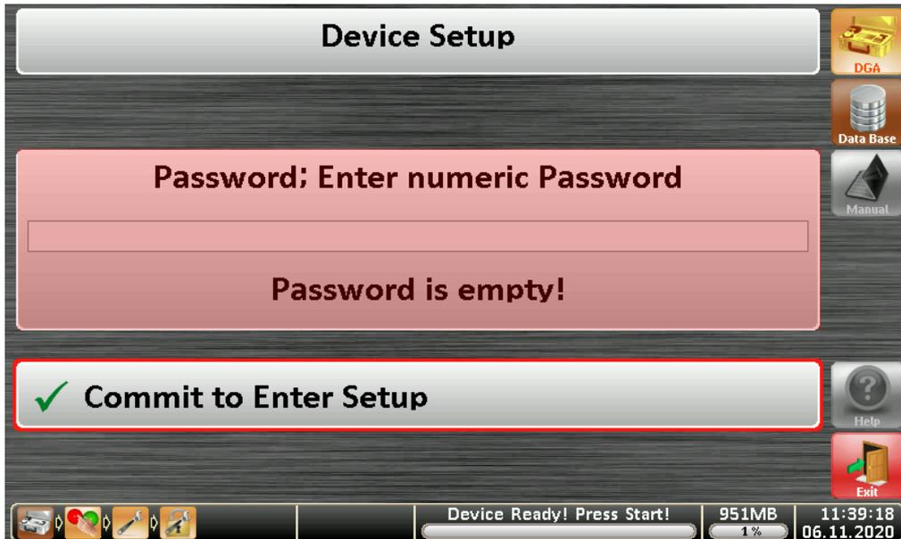
Now the password can be entered via the numeric keypad. The default password is 999. The password can be changed see [4.4.3.6].
