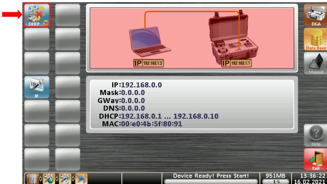
The configuration scheme is shown in the upper middle field. The lower middle field shows the assigned configuration data.
