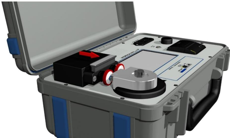
After it is released, the sliding block of the connection device is automatically brought into the starting position by spring pressure.
