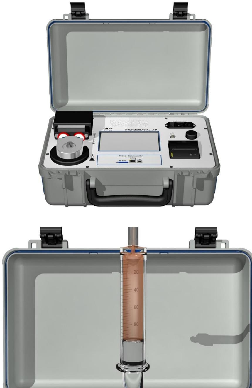
Fill the supplied oil sample syringe with 100 ml of the oil sample.
