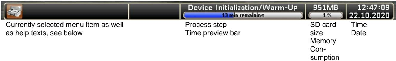
When a field is pressed, a help text appears in the left-hand area; the length of the display can be set individually, see [4.4.3.3].
