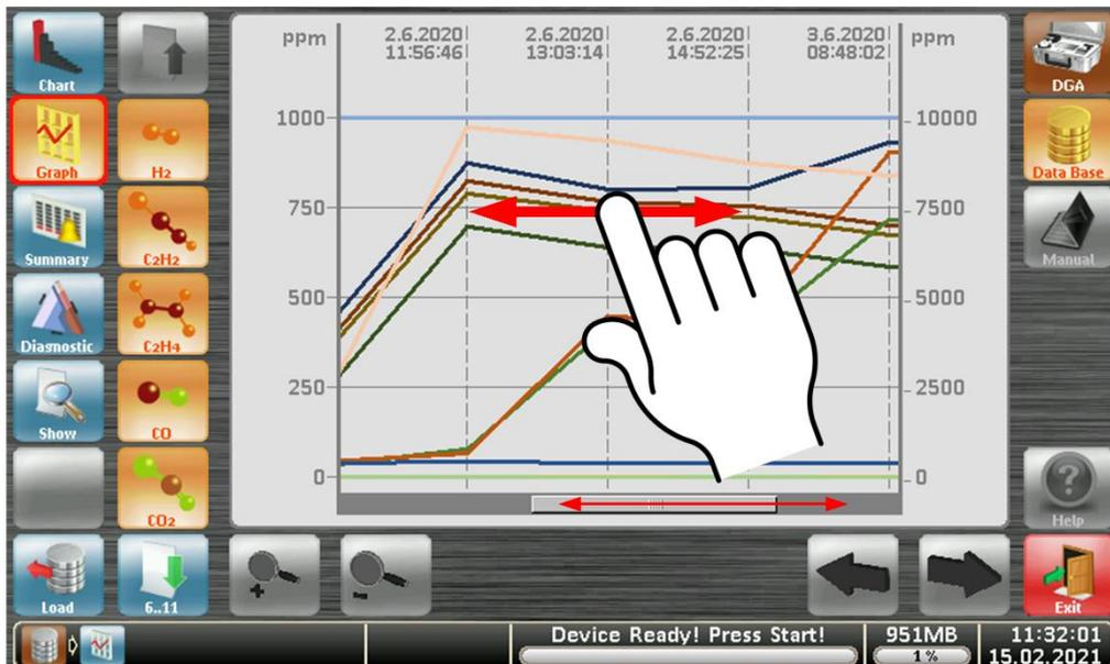
By pressing the control fields of the gases, gases can be hidden and shown again. This offers the possibility to show only those gases in the line graph that are important for the respective observation.
