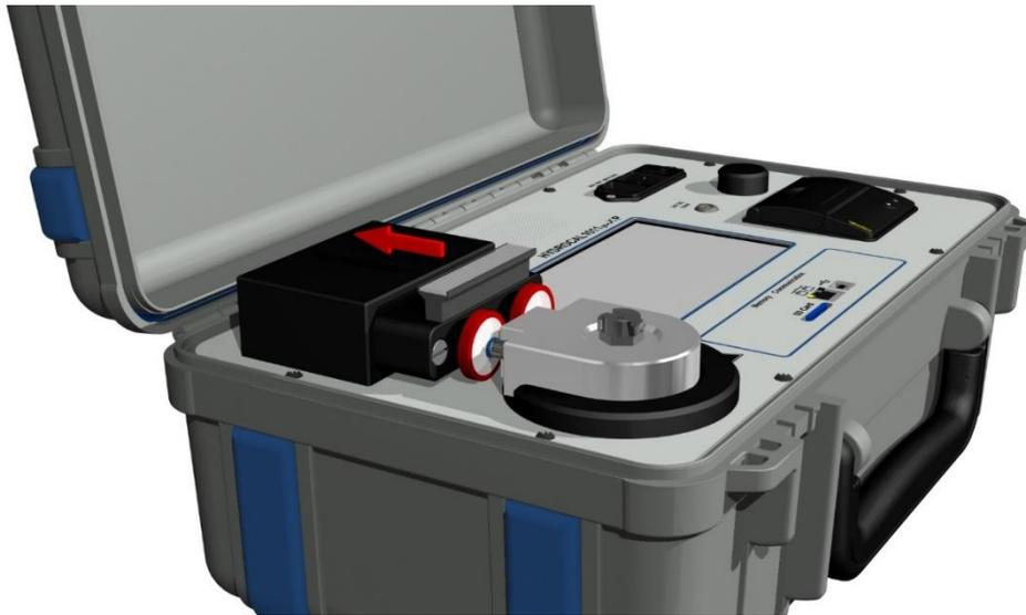
With the sliding block pushed back, pull the oil container out of the HYDROCAL 1011 *genX* P.
