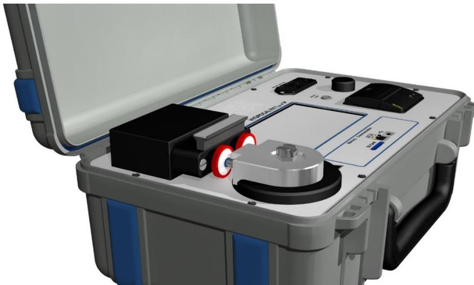
Push the sliding block of the connection unit back as far as it will go and hold it.
