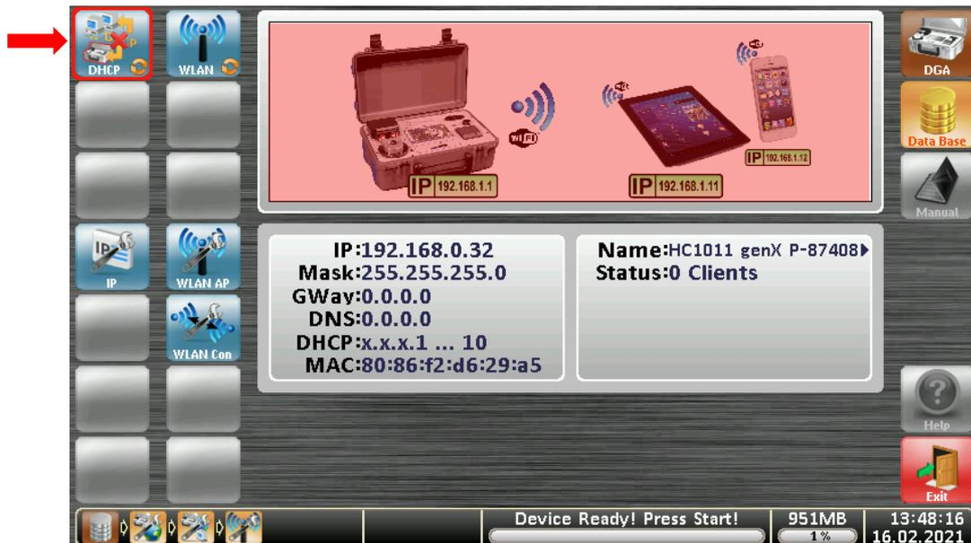
The configuration scheme is shown in the upper middle field. The lower middle fields show the assigned configuration data.
