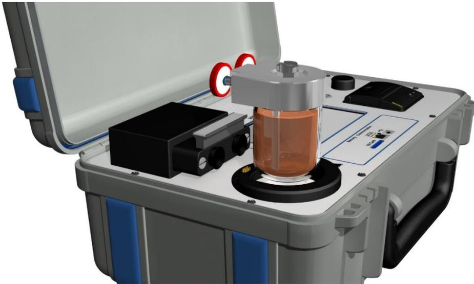
Unscrew the oil reservoir in the direction of the arrow
