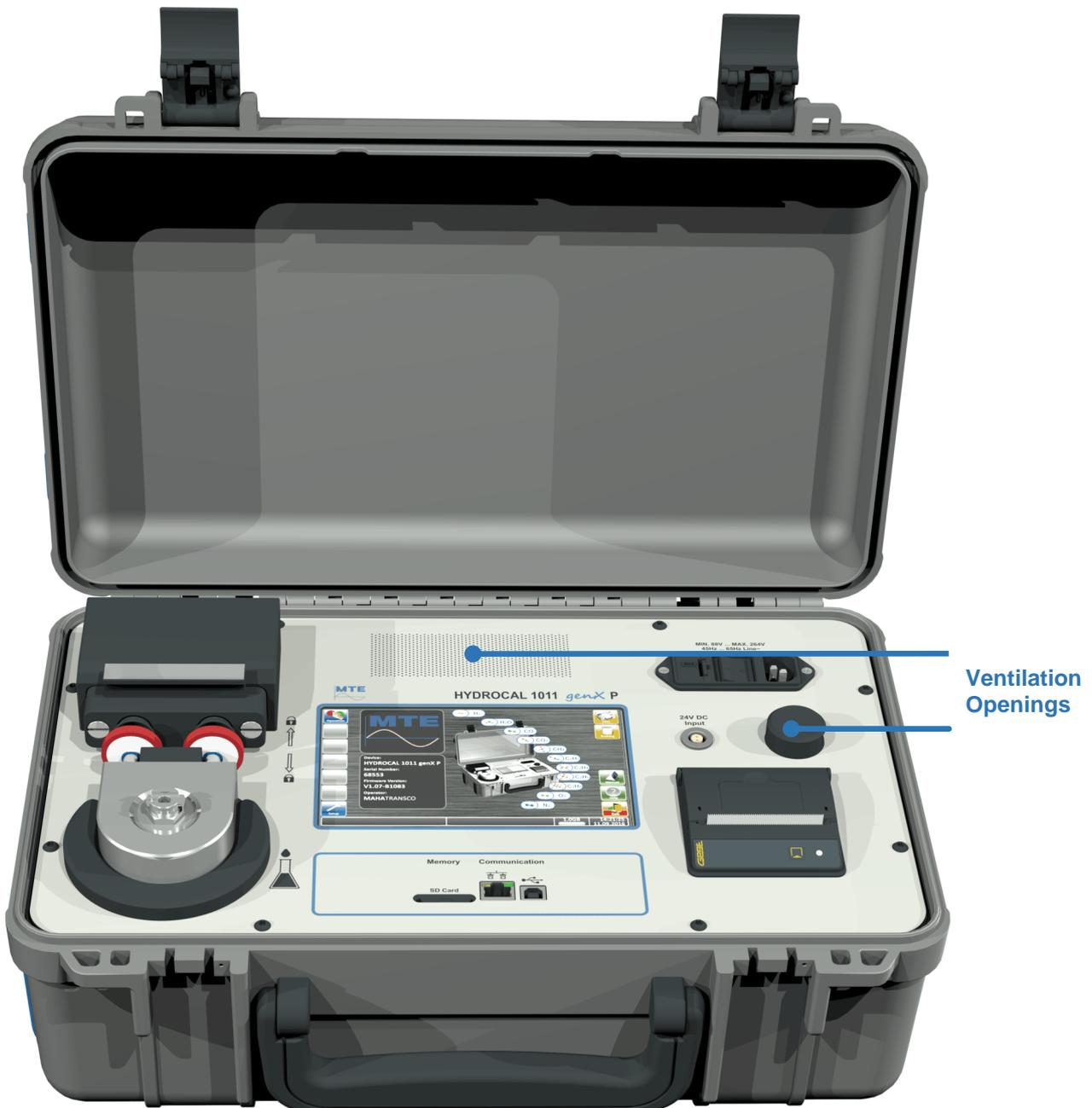
**Note:** The ventilation holes must always be kept free to ensure air/gas exchange. Do not cover or block the ventilation holes.
