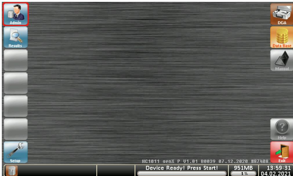
In the database menu, the stored results can be displayed and the basic settings of the device and the customer can be made.
